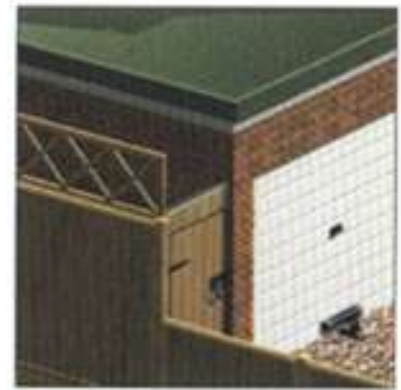
Locked side gate, not recessed
